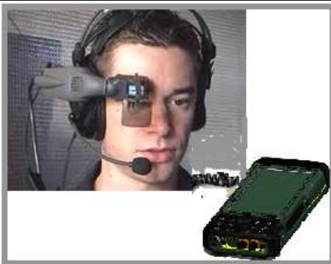
DB6 as pocket box computer for Military night vision and video recording On internal SSD for later review
