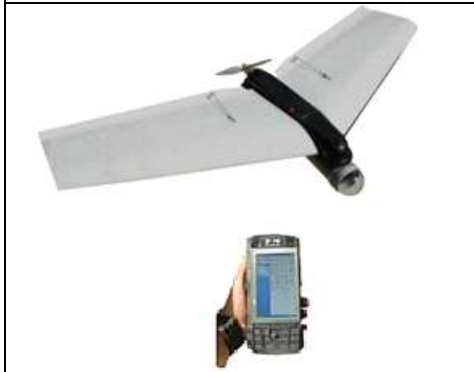
DB6 controls UAV & Receives Video from Camera for display & storage
