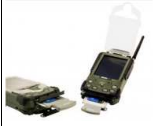
Plug in PCIe 34 card or your custom card With custom connectors if needs to (C.P)
